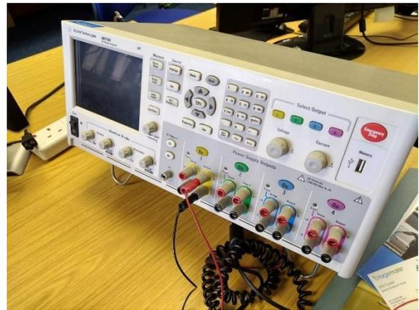
Figure 13 - Power Analyser used during power testing
