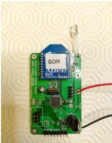
Figure 2 - Gen4 Probe Head Unit Prototype, with onboard XBee
