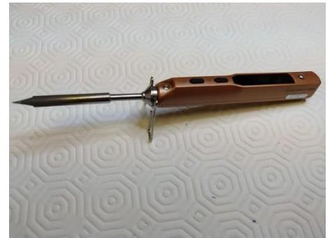
Figure 6 - Soldering Iron with fine tip
